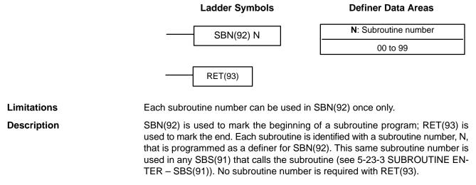
All subroutines must be programmed at the end of the main program. When one or more subroutines have been programmed, the main program will be executed up to the first SBN(92) before returning to address 00000 for the next cycle. Subroutines will not be executed unless called by SBS(91).
